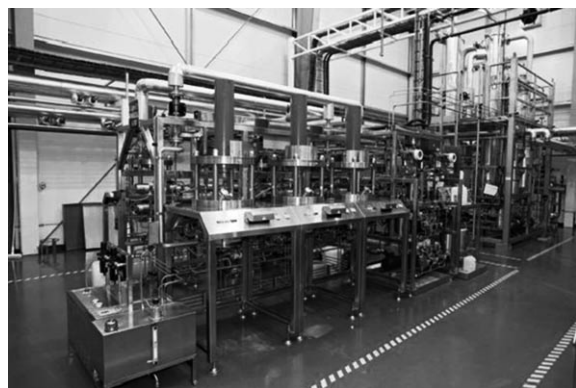
Figure 2. View of a production-scale SMB plant. Reproduced with permission from R.-M. Nicoud (Novasep, Vandœuvre-les-Nancy, France).
